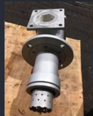
带内保温的热风烧嘴 Internal insulated Burner for Hot Air
