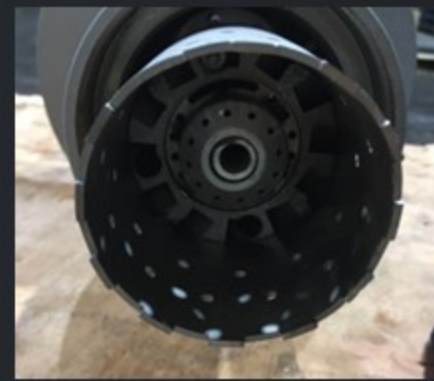
带内保温的热风烧嘴 Internal insulated Burner for Hot Air
